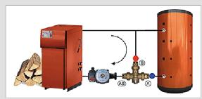
Mounting in mixing mode with anti condensing function.
