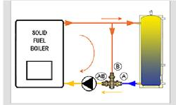
At the achievement of the opening temperature (f.i. 55°C), the way to users (gate A) proportionally starts to open meanwhile, the by-pass (gate B) is going to be closed. The boiler temperature slowly rises, giving energy to the user but, in any case, it will not decrease any more below the calibration temperature (f.i.55°C).
