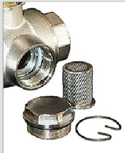
The stainless steel filter placed inside the ball can be easily removed, to be cleaned and inspected, while the valve is in closed position. The ball valve can be installed either with or without the filter (in this case the filter can be used for a limited time only, for example to clean the system).
